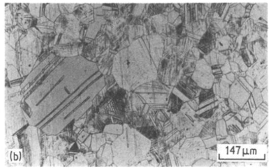
Figure 3 Optical micrographs (a) ST; (b) 36% CW; (c) 72% CW.
